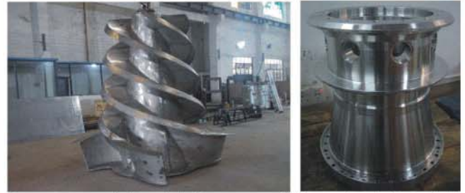
Screw conveyor shaft material is stainless steel-1
