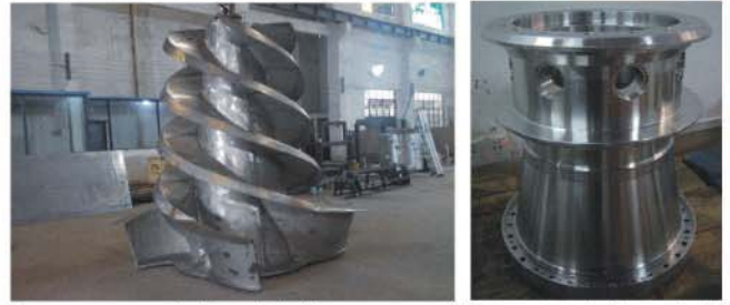
Screw conveyor shaft material is stainless steel-1
